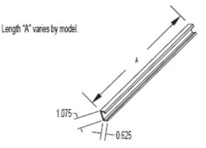
2. The channel assembly will provide infinite vertical and horizontal adjustment and not limit the positioning of shelves or panels. All mounting hardware will be furnished.
